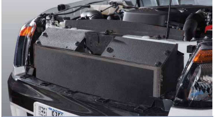
Radiator and battery protection
